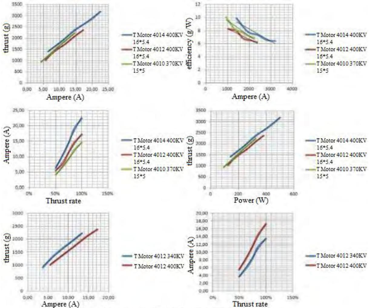
Figure 5: Comparison of chosen T Motor among the other T motors
