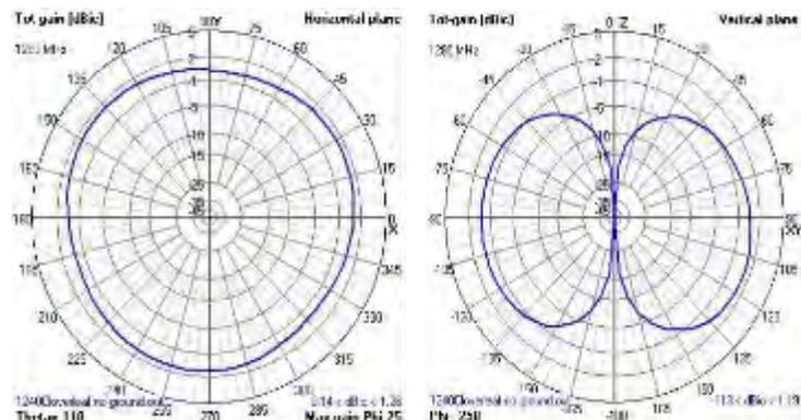
Figure 11. Cloverleaf antenna and its radiation pattern
