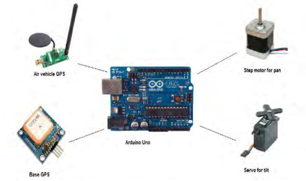
*Figure 8. Electronic design of Antenna Tracker*
