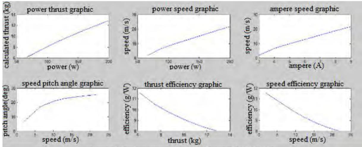
Figure 4. Performance graphs of T Motor MN4012 400Kv
