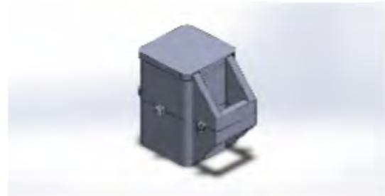
*Figure 6. Airdrop release mechanism*
