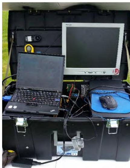
*Figure 8: Portable Ground Control Station*
