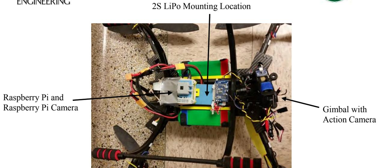
*Figure 5: Payload Mounting Plate in Mission Configuration*
