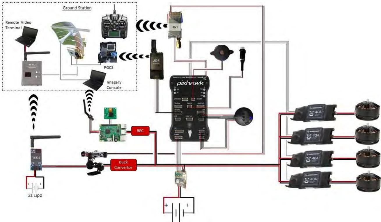
*Figure 6: Complete System Architecture*
