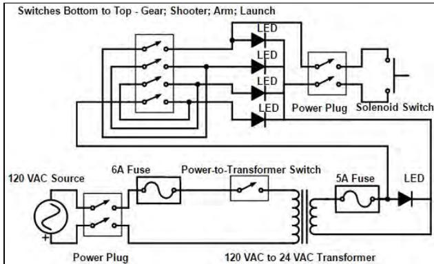
**Figure 3: Launch box wiring schematic**
