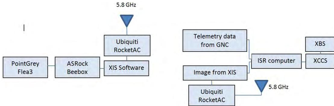
**Figure 9: ISR System Diagram**
