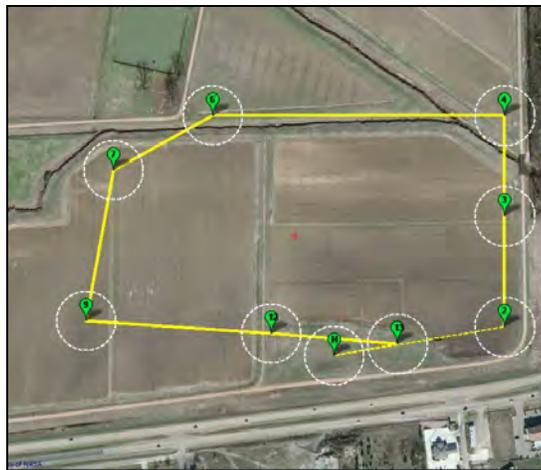
Figure 10: Autonomous Mission Plan
