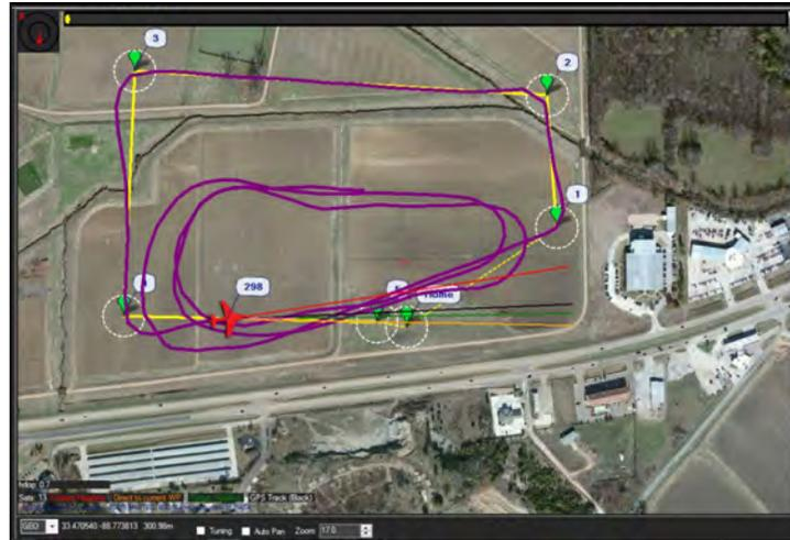
**Figure 11: Autopilot Tracking After Tuning**
