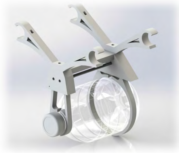
Figure 13: A render of the bottle drop mechanism.
