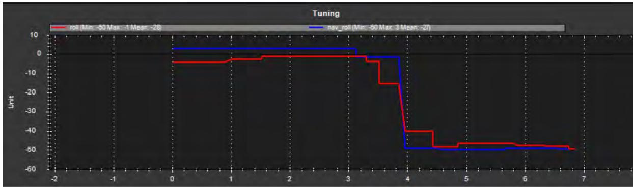
**Fig.13. Actual Roll (red) and Commanded Roll (blue) v/s Time:** The response curves for the roll axis showed the actual attitude following the demanded attitude closely. Response times were minimized to allow for optimum tracking without exceeding the structural limits of the airframe.
