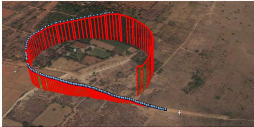
**Fig.9.** A plot of the UAS’s position during an autonomous landing sequence showing an ideal glide slope and control over positioning.
