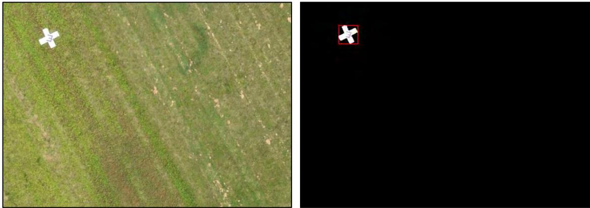
**Fig. 5. (A, B) Selection of potential targets:** An example of the output result (**Fig. 5.B**) after the original image (**Fig. 5.A**, here, shown as a cropped version of the original image to highlight target) is passed through Saliency Detection and the aforementioned Filters.
