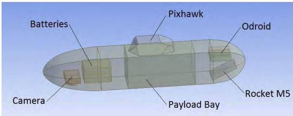
Figure 2: Fuselage sizing and Payload arrangement
