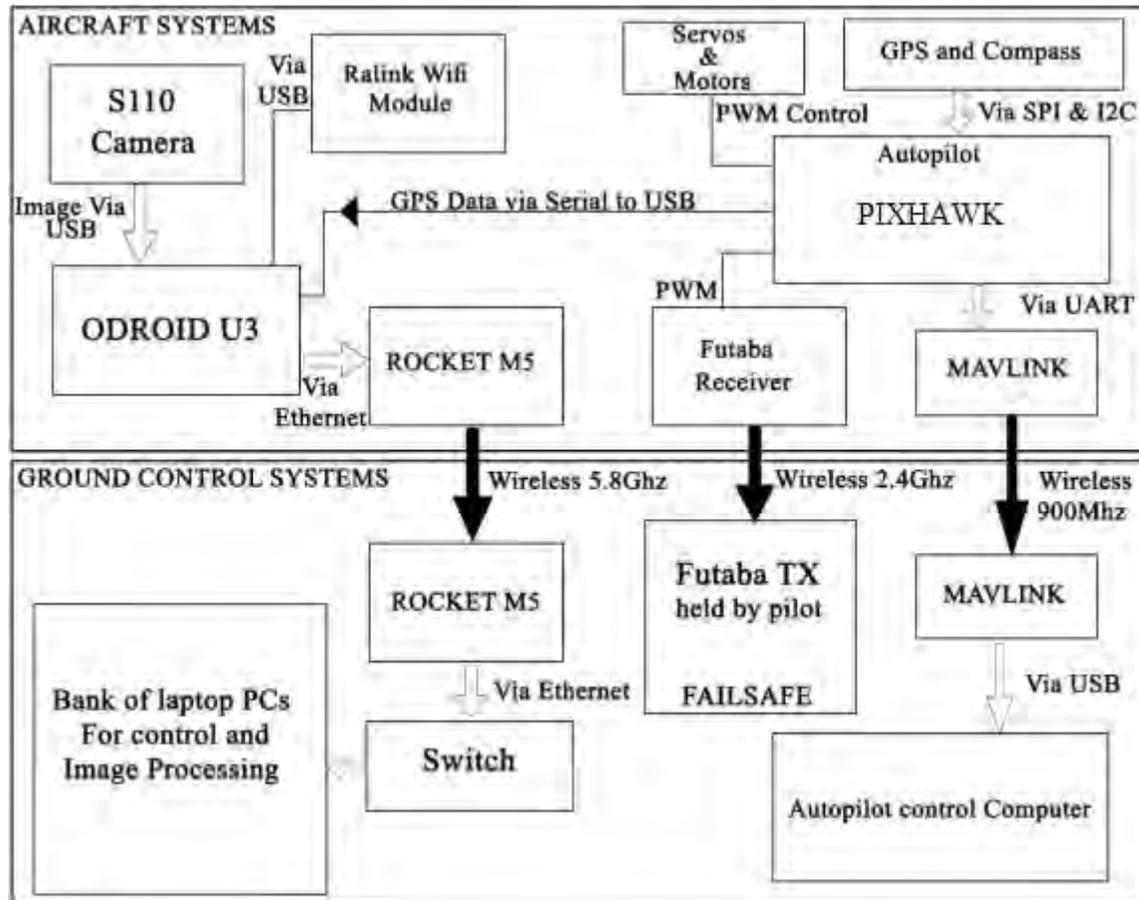
Figure 4: High - Level Block diagram of the System
