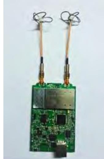
Figure 6: Cloverleaf antennae on the Plane
