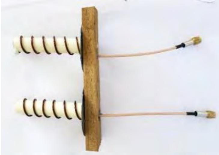
Figure 5: Helical antennae at the Ground Station
