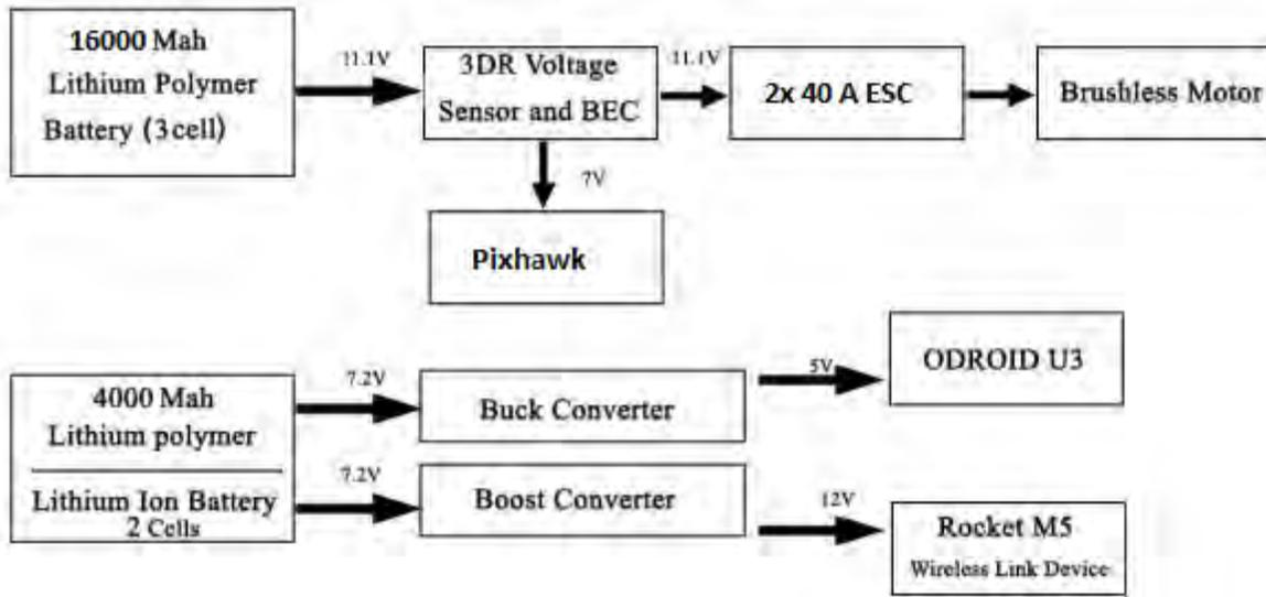
Figure 3: Power Systems Block Diagram
