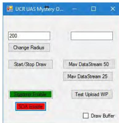
**Figure 2.7.6** Custom GUI to enable and disable eggdrop, SDA, and various other parameters. Green means enabled and red means disabled.
