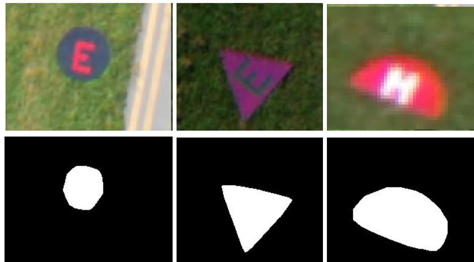
Figure 2.7.5 Image processing using color segmentation
