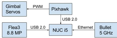
Figure 2.4.1 High level block diagram of the payload system
