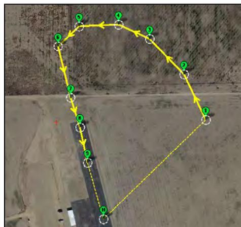
**Figure 2.7.2** Autonomous landing sequence scenario with wind from south to north
