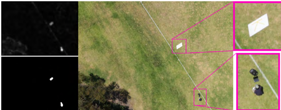
Figure 9: Salient object detection finds emergent target “Eric” and a painted plywood target during an imaging test flight.
