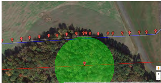
Figure 7: Path between two waypoints that avoids an obstacle. The mission is last year’s competition.
