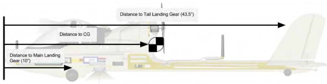
Figure 4: Location of CG for the Penguin (arrows & labels were drawn on the image from the Finwing Penguin Manual [1]).
