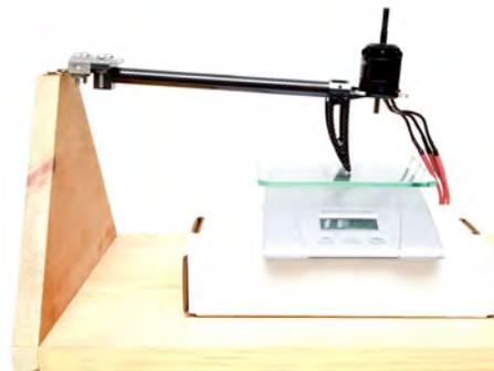
Figure 10: Static Motor Test Mount.
