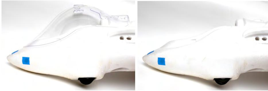
Figure 3: (Left) Fuselage with Canopy. (Right) Fuselage without Canopy.
