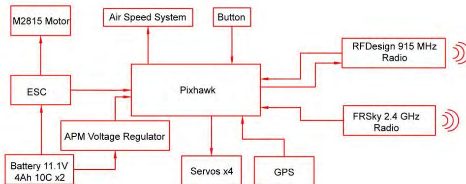
*Figure 6: Autopilot Block Diagram.*
