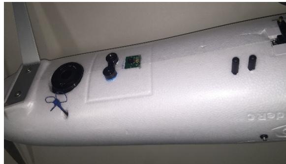
**FIGURE 5 – SENSOR AND ANTENNA POSITIONS**
