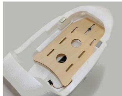
**FIGURE 2 - ADJUSTABLE FUSELAGE TRAY**
