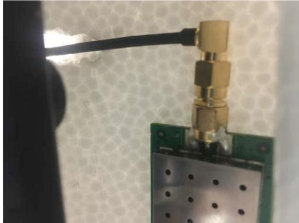
**FIGURE 9 – BULLET CONNECTOR MODIFICATION**
