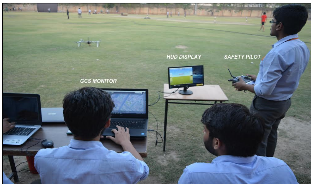
Fig. 8- Ground Control Station Setup with HUD for safety pilot
