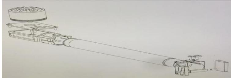
(Figure 2.2 - Expanded image of quadcopter arm)
