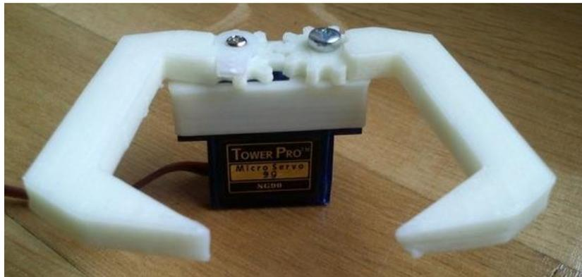
Figure 6: Representation of the payload drop mechanism
