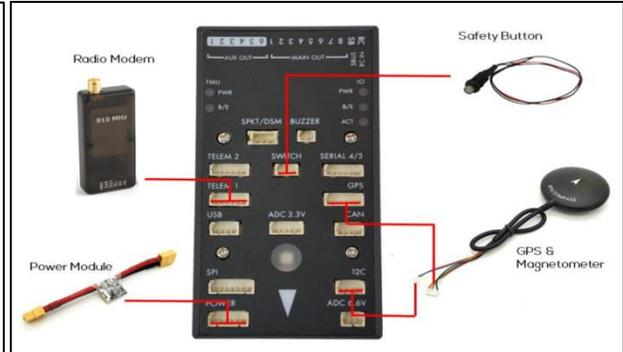
Figure 3: Pixhawk Connections (2)
