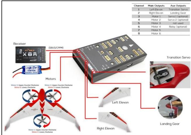
Figure 4: Pixhawk Connections (1)
