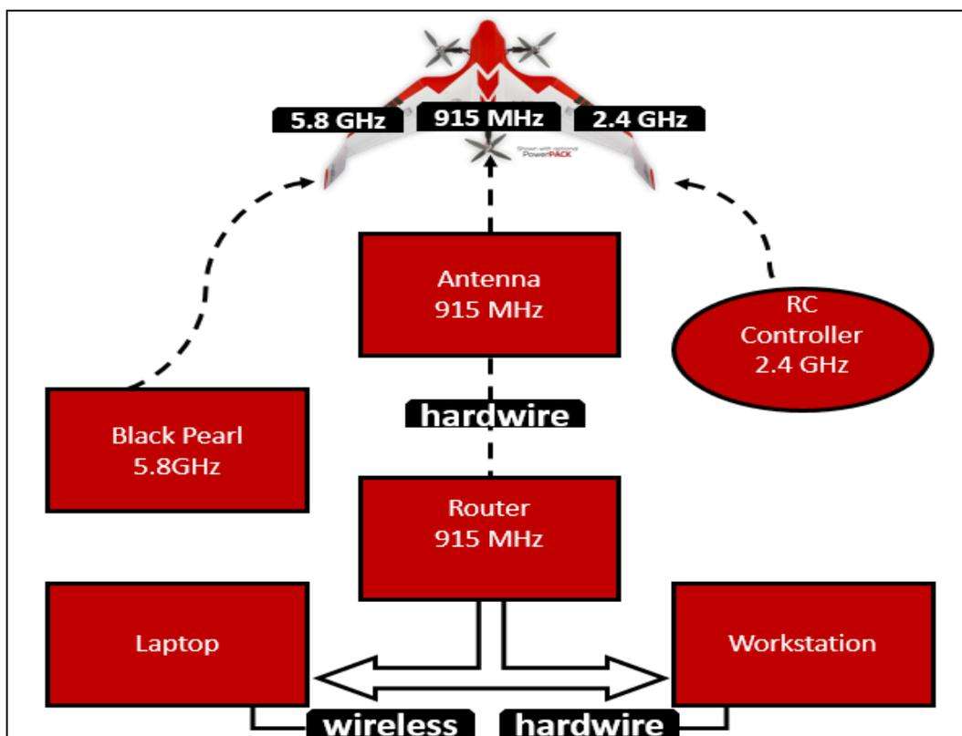
Figure 7: Ground Station Block Diagram
