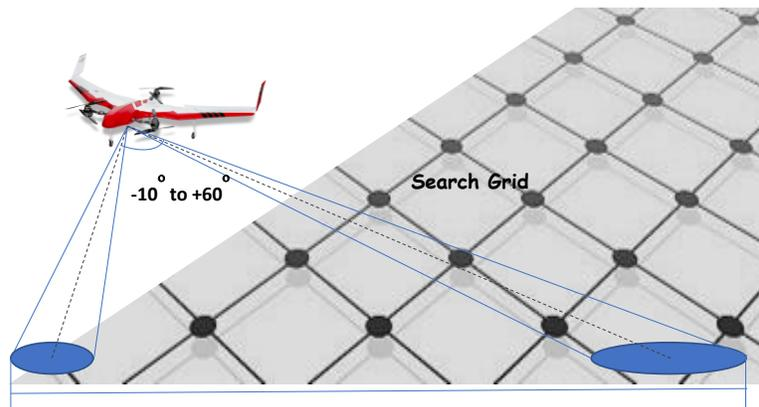
**Figure 6: Camera FOV Diagram**
