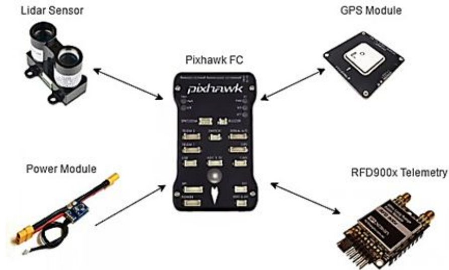
Figure 2.2 Pixhawk Sensors and Telemetry
