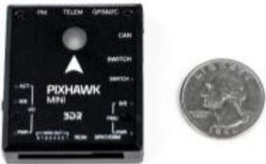
A sample picture of the PixHawk Mini control board, next to a quarter for size comparison.<sup>2</sup>
