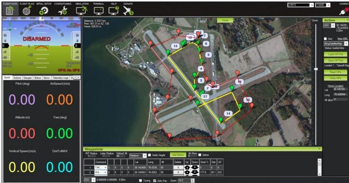
Figure 2-7: Image of primary Mission Planner Interface with example Flight Mission.
