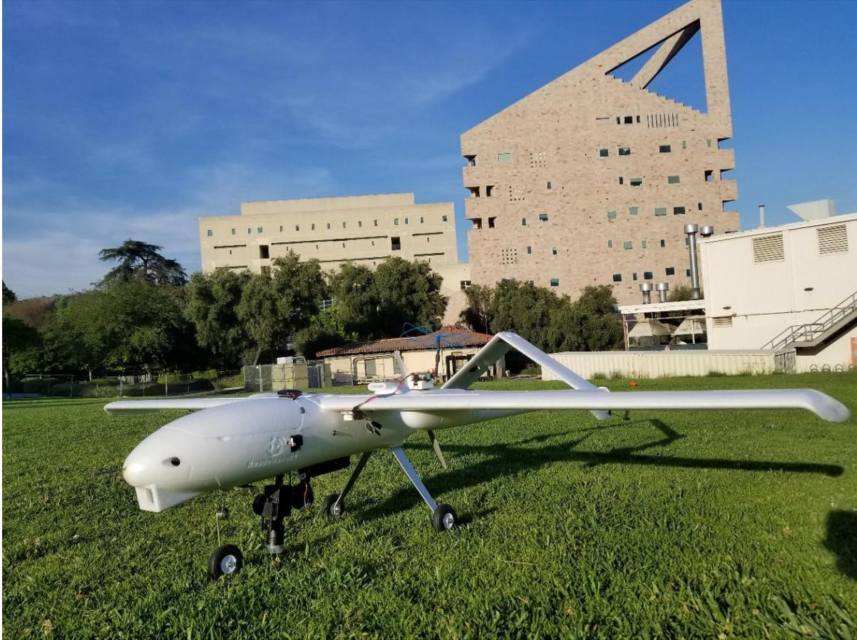
**Figure 2-1: Picture of the RMRC Anaconda UAS that will be used in AUVSI-SUAS competition.**
