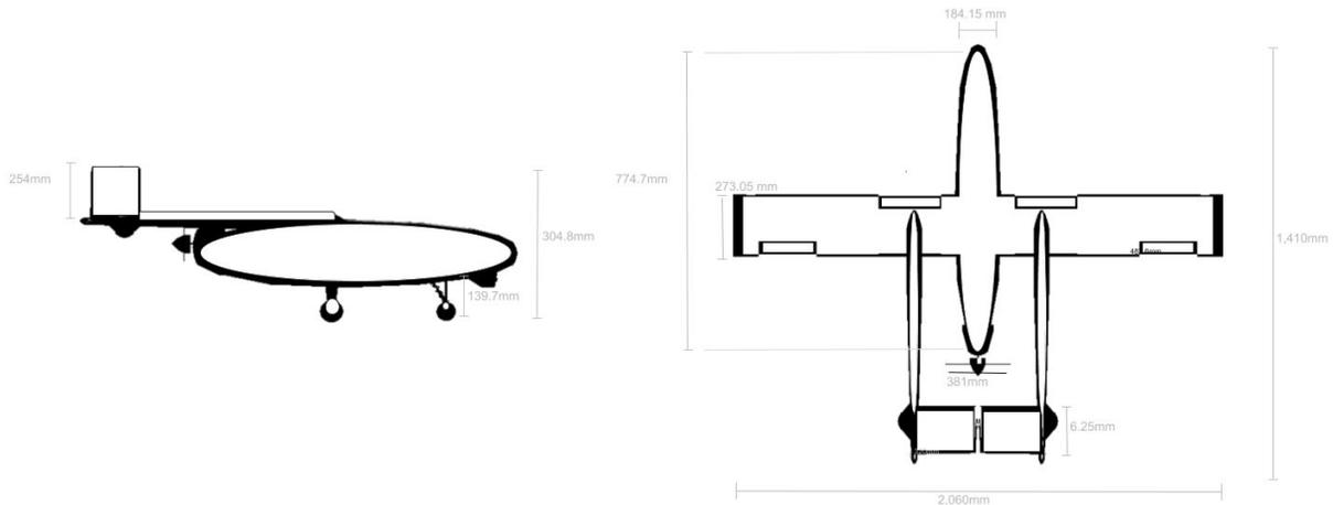
Figure 2: Specification View and Measurement of the Plane
