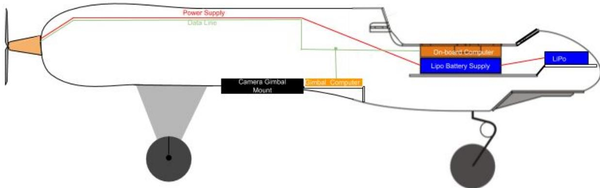
Figure 4: Specification of internal Hardware Placement (RMRC Anaconda)
