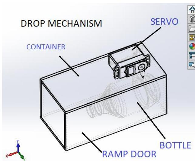
Payload Drop Mechanism
