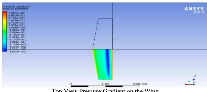
Top View Pressure Gradient on the Wing
