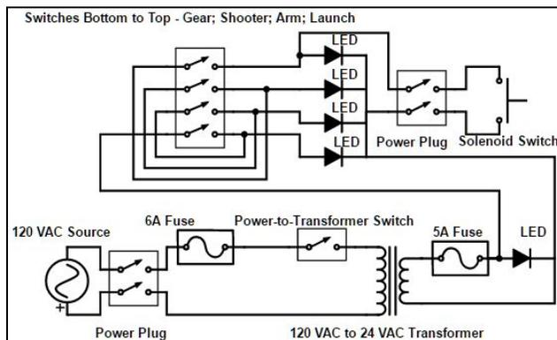
**Figure 7: Launch box wiring schematic**
