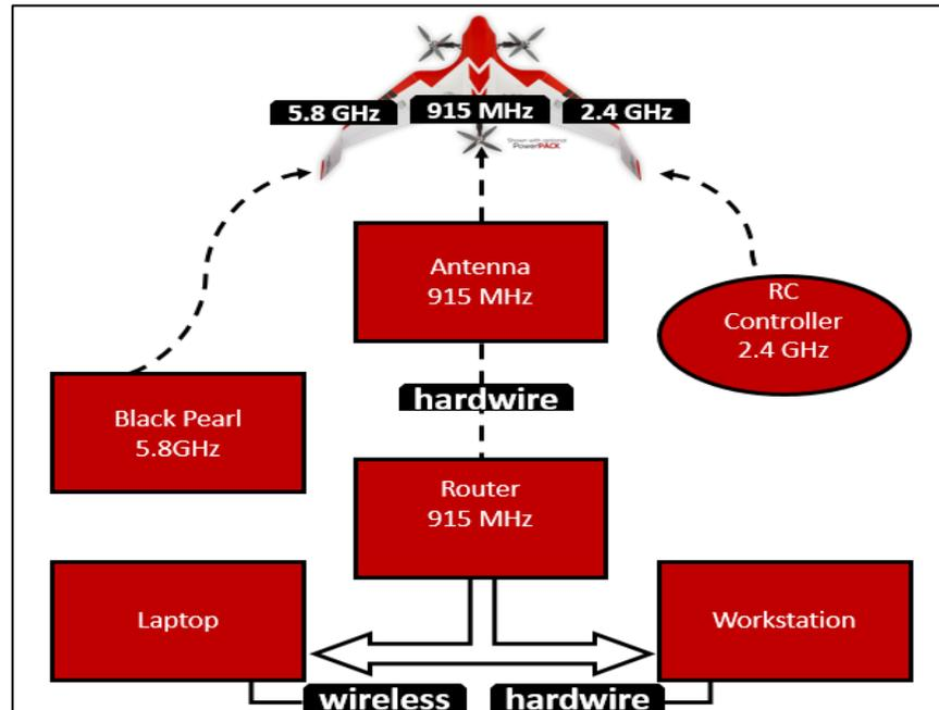
Figure 4: Ground Station Block Diagram
