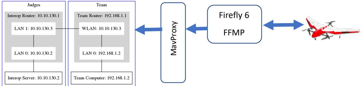
**Figure 1.** Interoperability network topology. Figure adapted from [1]
