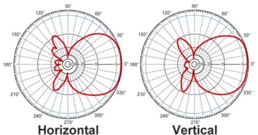
Figure 6: HG980P Beam Patterns
