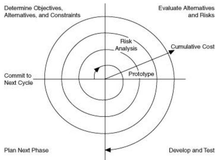
Figure 1: Spiral Model for iterative development
