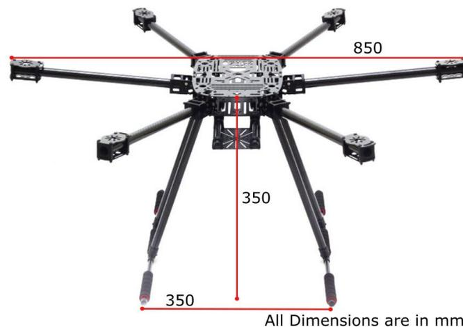
Figure 2: Dimensions of the Hexacopter
