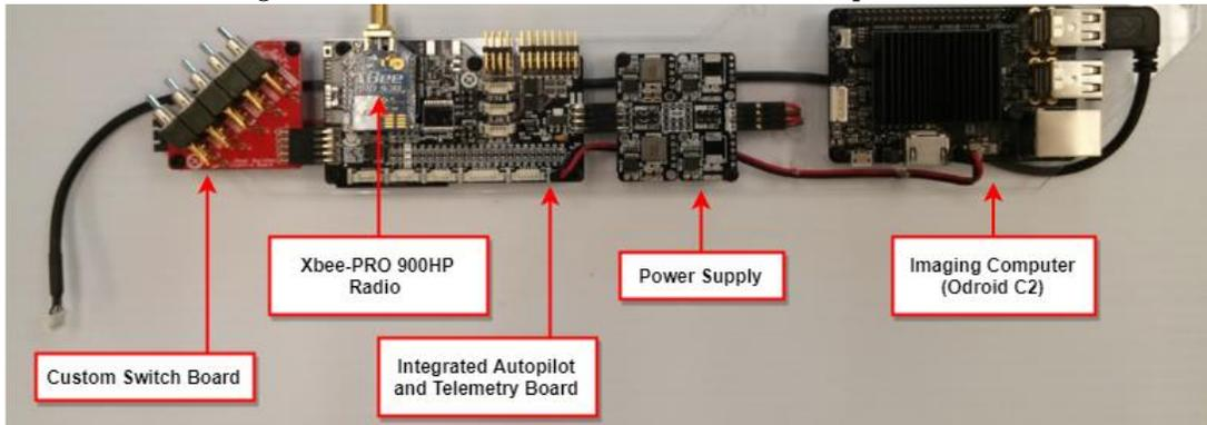
Testing of the electronics began with ground tests to check the status of the telemetry link, RC link, PWM servo output, IMU output and power supply. This is depicted in Table 3.
