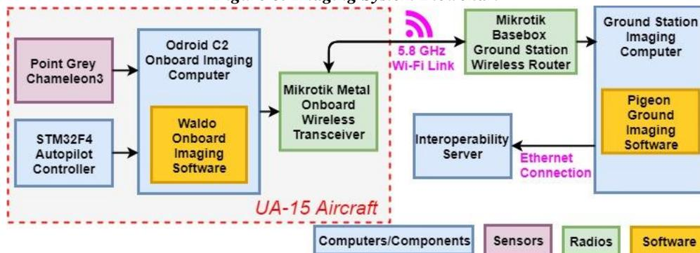
The imaging system consists of:
