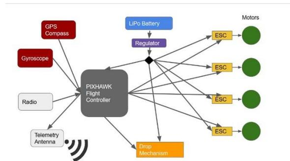
Figure 1 - Wiring Diagram for a 4 rotor UAS. Much of the wiring, apart from the motors, is identical to the 8 rotor UAS
