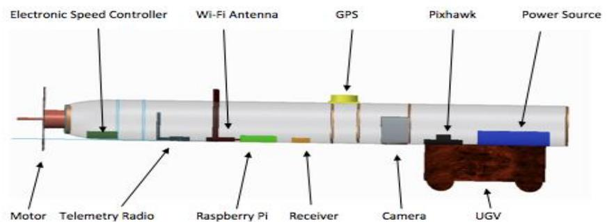
Figure 3: Fuselage Layout
