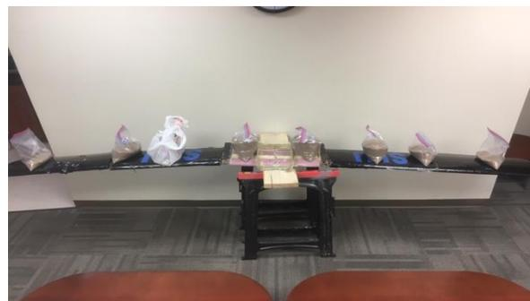
**Figure 4: Wing Loading Test**
