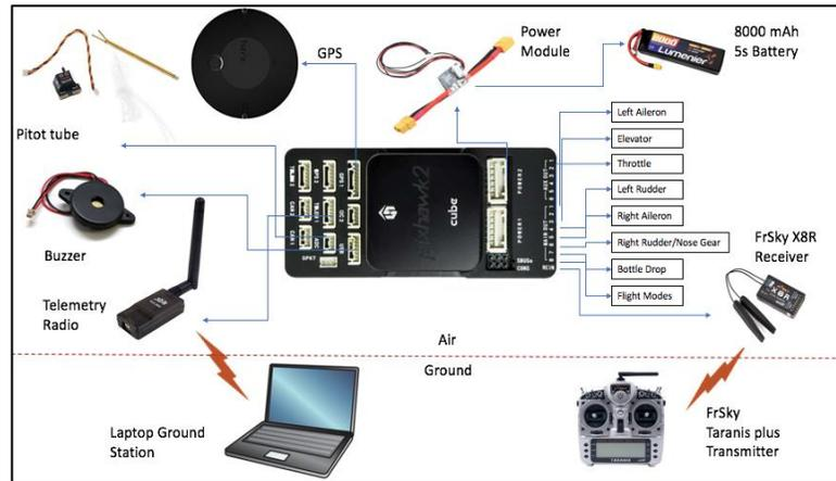
Figure 5: Pixhawk Schematic
